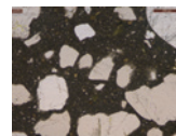
Fig 1: AALBORG EXTREME® in normal light mode at x100 magnification. Aggregates are white areas whereas cement paste is darker-brownish areas.
